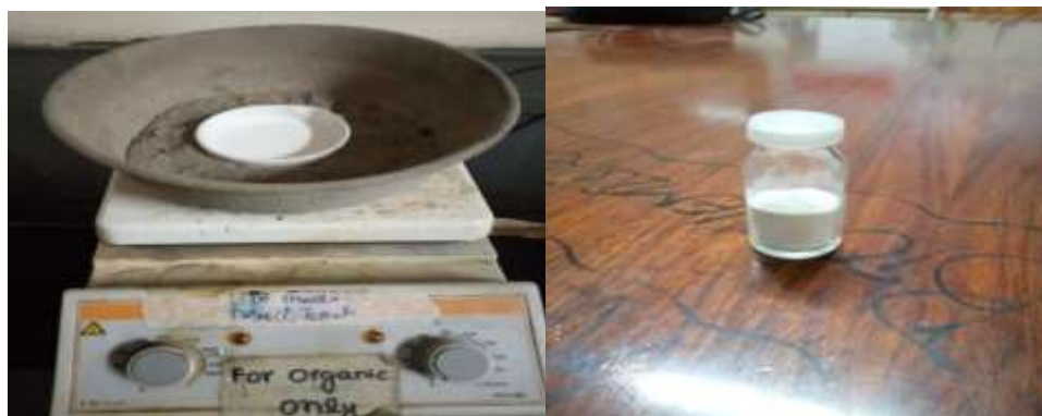
Figure 3.4: Open atmosphere annealing of TiO 2 at 300 °C and Prepared TiO 2 nanoparticles
