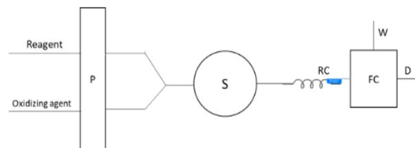
Figure 2: Scheme of the employed flow system, P: peristaltic pump, R.C: reaction coil, S: sample injection, W: waste, FC: flow cell
