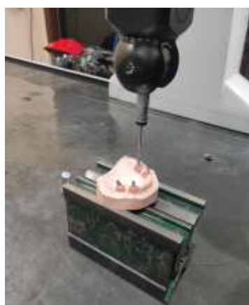
Figure 9: Stone cast being measured with standard abutments in place on the CMM machine. CMM: Coordinate measuring machine
