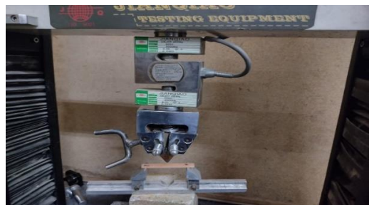
Figure (2). Universal Testing Machine and the specimen in the test
